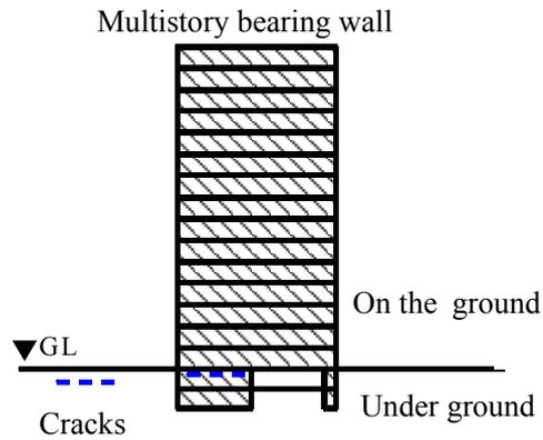
Figure 8 Schematic illustration of multistory bearing wall with large opening at basement
