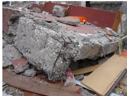
Photo 19-2 Foamed polystyrene contained in concrete
