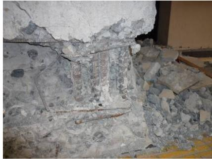
Photo 20-4 Bar arrangement in wall edge
