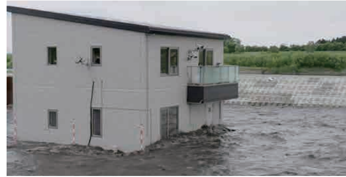
実大木造住宅の水理実験 Hydraulic test on full-sized wood house
