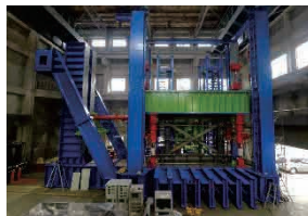
鉛直方向・水平2方向加力装置(09) Vertical and horizontal 2-directional force application device
