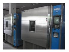
Chamber of Programing for temperature and humidity
