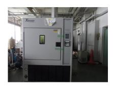
Ultraviolet accelerator facility
