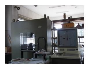
500t strength test machine with high rigidity
