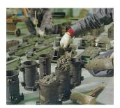
Schematic concrete specimens making
