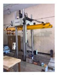
Dynamic loading-deformation testing machine
