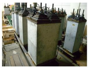
Creep Compression Test of High Strength Concrete Columns
