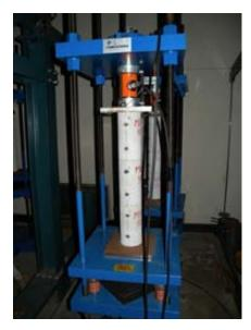
Creep Compression Test of Cylindrical Concrete Specimens
