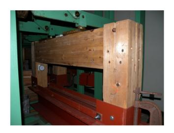
**Creep Test of Timber Joints**
