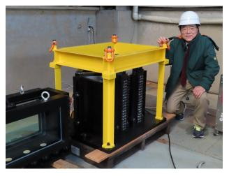
Shear box for the centrifuge
