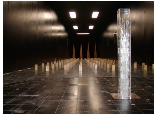
WIND PRESSURE TEST ON A MODEL OF A SKYSCRAPER
