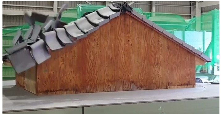
ROOF TILE SCATTERING EXPERIMENT
