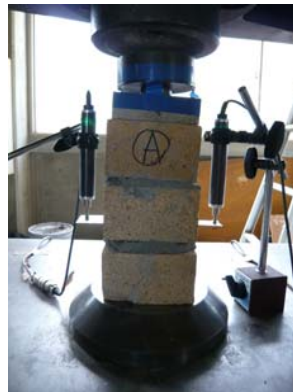
Compression test of prism specimen
