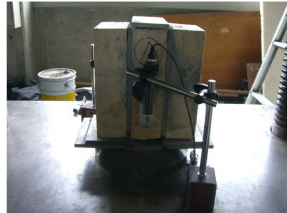
Shear test of mortar joint
