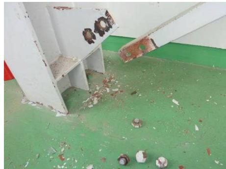
Photo 3.50 Fracture of Bolts
