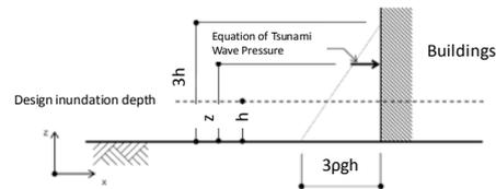
$$\text{Equation of Tsunami Wave Pressure: } q_x = \rho g (3h - z) \quad (1)$$
