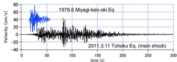
Fig.2.7 Comparison of the Recorded Motions at the 1<sup>st</sup> floor of Tohoku University Building between 1978 Miyagi-Ken-Oki and 2011 Tohoku earthquakes
