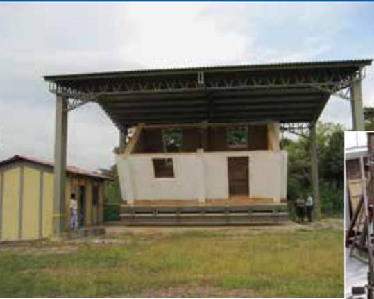
An improved adobe structure was successfully tested on the incline platform built at the University of El Salvador.
