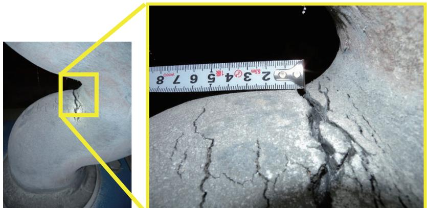
Photo 9.2-17 Lead damper and cracks on the surface
