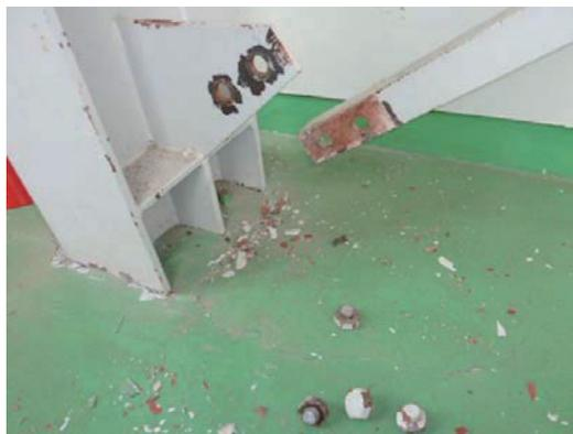
Photo 6.4-4 Fracture of bolts
