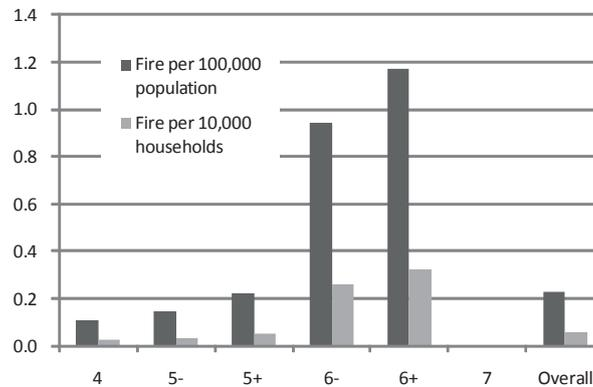
Fig. 8.3-1 Relation between break-out ratio of fire due to earthquake motion and seismic intensity
