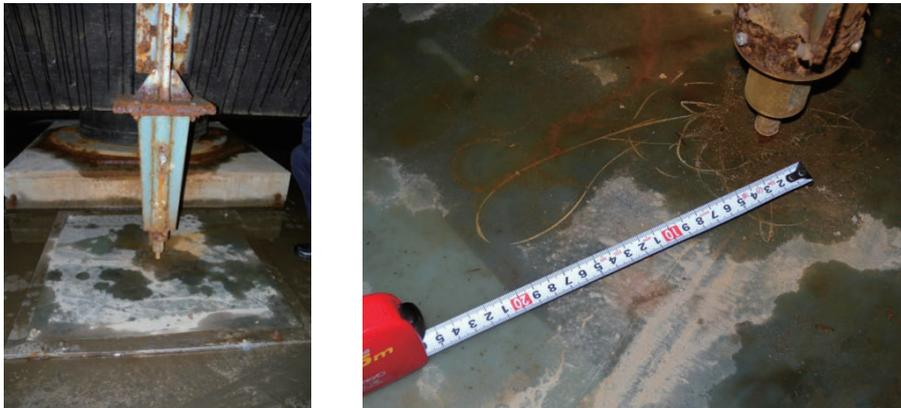
Photo 9.2-11 Trace of displacement of the SI floor on the scratch board
