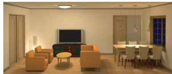
Mood example 2: Relaxing, etc. (ceiling light 70% + floor lamp on low + 1 pendant on)
