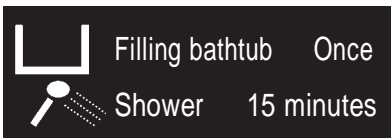
Fig. b Detailed display of remaining hot water level
