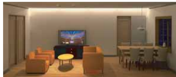
Mood example 2: Watching a movie, etc. (down light x 2 + indirect lighting 50%)
