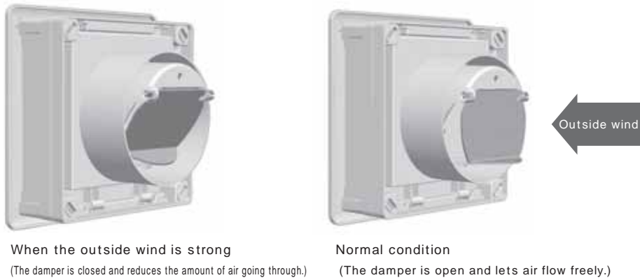
Fig. 7 Example of air vent with damper preventing interference from outside wind
