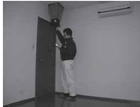
Fig. 10 Airflow rate measurement being performed
