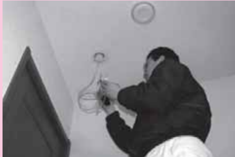
Fig. b Example of indoor air terminal device designed for k-factor method and actual measurement being taken
